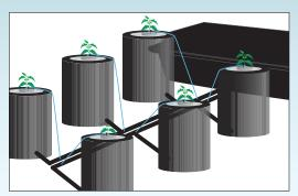
Cycle your system and visually ensure that the nutrient solution level coincides with the placement of the root zone. This is critical for success.
