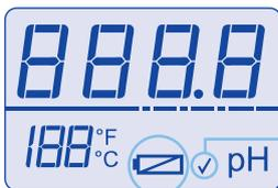
**Check mark/tick to indicate successful pH calibration**
