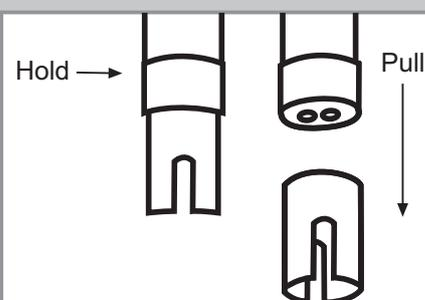
Figure 5. Shroud Removed
