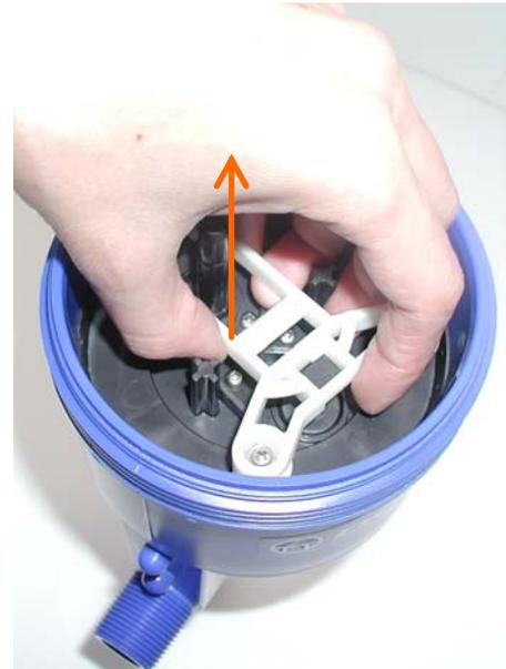
Insert piston into the body half way down, suspend the unit from the valve support **ONLY**, then lift it. The piston should be snug in the body and the body should not fall off. If it does, the piston shell needs to be replaced. Also inspect the inside of the body and look for deep vertical scratches. If this is the case, the body needs to be replaced.
